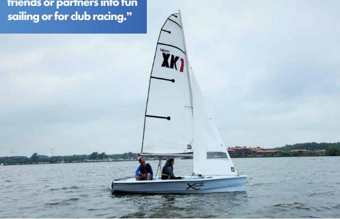
The first rota-moulded keel boat and the reason we chose the boat from our range, was because of the beautiful hull shape, which really suited the concept of being designed for hiking. The incredible beam, measuring in at 2m wide, makes for a very comfortable, spacious and uncluttered cockpit. This impressive design allows the crew to easily control the XENON XK1, which has a smaller rig than the standard XENON for ease of handling with the keel version.
