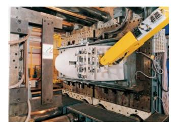
**Pictured Above** is a photograph of the Topper in production using the previous injection mouldng techinque.
