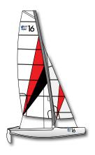
Length: 4.72m Beam: 2.25m Total Rigged Weight: 140kg
