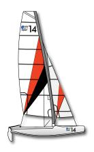
Length: 4.25m Beam: 2.05m Total Rigged Weight: 110kg
