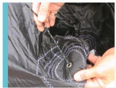
Temporarily remove the red ball from the Gennaker halyard. Then pass the end of the Gennaker halyard through the eyelet in the sail as shown.
