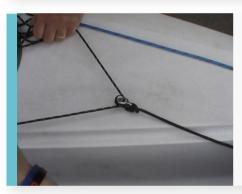
Take the free end of the halyard through the pulley to pull the pole out; it is underneath the Gennaker chute, and it may need to be moved for the pulley to be exposed.
