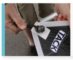
Then tie the Gennaker pole line to the TACK of the spinnaker, you can either use the ball and loop method or a bowline loop.
