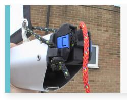
Pull on the red reefing line so that it comes out of the boom some way.
