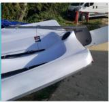
For launch and recovery the rudder should be left attached, with the blade lifted up and held by the uphaul line locked in the small cleat on the top of the tiller arm.
