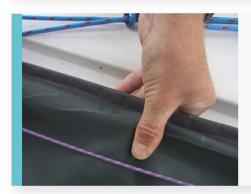
Pass the line up the chute, feeling for the ball inside, until it reaches the opening at the front.
