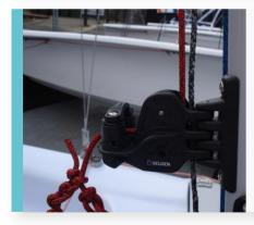
Having fixed the boom and gnav to the mast you can thread the gnav control line.
