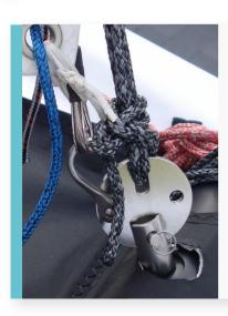
Attach the foot of the jib to the shackle in the rear hole of the disk in the furler at the front of the boat (Ensure the furler is fully wound up.)
