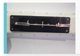
The keel locking mechanism front and rear MUST be fully secured with the pin to lock the keel in place and stop movement of the keel.
