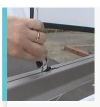
As the cleat is at the base of the mast you can sweat the halyard in order to make sure that the sail is at the top of the mast.
