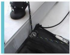
Take the other free end of the halyard and take it through this pulley on the front of the cross beam. 2
