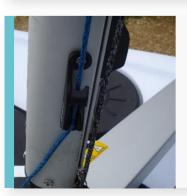
Cleat the main halyard in the cleat on the left of the mast.
