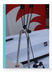
Attach the boom onto the mast with the pin on the lower of the two fittings.
