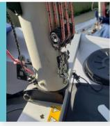
Once the keel has been lowered fully, the pulley system can be removed and attached to the eye at the base of the mast (toward the bow) for storage.
