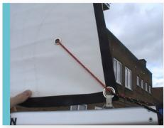
Feed the reefing line through the eyelets in the leech of the sail.
