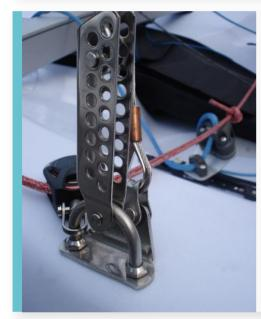
Untape all the ropes attached to the foot of mast. Attach shroud adjusters to the shroud eye each side - approximately the 7th hole down (approximately the middle of the adjuster). Subsequently, you can attach at the captive pin on the base of the plate.
