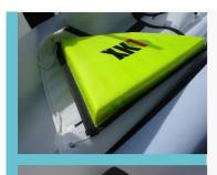
Tie the flotation panel to the top of the mainsail by passing the white lines through the eyelets in the sail and secure with a figure of eight knot. 1
