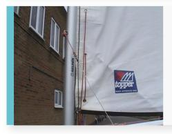
Release the main halyard from the cleat, and uncleat the Gnav, and then pull on the reefing line.
