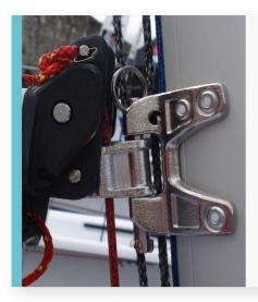
Attach the boom onto the mast with the pin on the lower of the two fittings.
