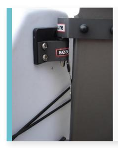
When the Rudder is attached ensure that it is fully engaged on to the pintle and gudgeon so that the retaining clip is able to spring out to hold the rudder in place.
