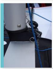
Fix the base of the mast to the mast step on the cross beam with the pin and ring from the mast step.
