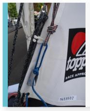
Pull the jib halyard in order to raise the jib (using the 2 part halyard attaching the plastic hanks as you pull the jib up to the forestay wire, and then feed the rope from the cleat through the loop in the halyard.
