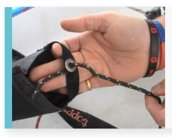
Pass the halyard through this eyelet in the bottom of the spinnaker chute
