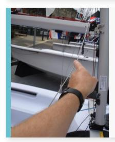
Now tie the lowers onto the fitting on the mast or on the hull (depending on the make of mast).
