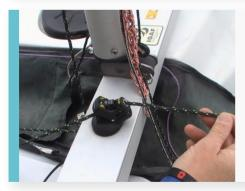
Take the halyard through the Spinlock cleat that is mounted on top of the crossbeam.
