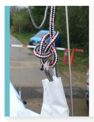
Tie the head (top) of the jib onto the jib halyard.
