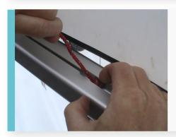
From the top eyelet, the reefing line comes back down to the boom. Tie a stopper knot in the end of the line, and then slide the knot into the cut out in the boom.
