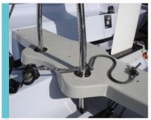
Thread the mainsheet. Starting from the centre cleat on the hull.
