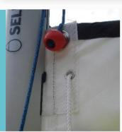
Raise the sail by placing the bolt rope in the cut out of the mast just above the boom, and then pulling on the halyard.
