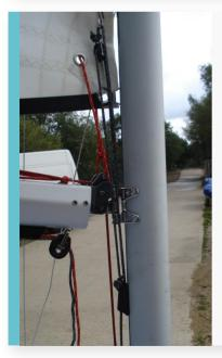
Cunningham - Take the tail attached to the gooseneck fitting and feed through eye in the sail then down through the cleat on the side of the mast.
