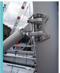
Next attach the strut to the upper fitting on the mast. Ensure the toggle is correctly orientated as per the Selden/Super Spars info sheet.
