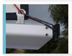
Pass the outhaul through the eyelet in the clew, and then back to the end of the boom, where the stopper knot end of the outhaul it fixed behind the lug on the boom end fitting.
