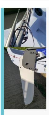
Whilst sailing the rudder should be locked fully down using the pulley system that cleats off on the side of the tiller arm. When you look over the back the rudder will appear to be tucked slightly under the hull, this is as it should be.
