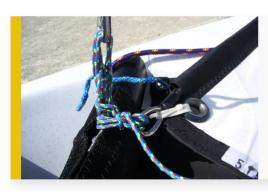
Then attach the foot of the jib to the eye at the front of the boat using the tail of the forestay.
