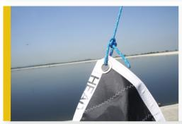
Follow the luff to the head of the gennaker (marked "H") and attach it to the top end of the gennaker halyard using a bowline. Pull the gennaker up the mast slightly to give yourself some slack in the downhaul.
