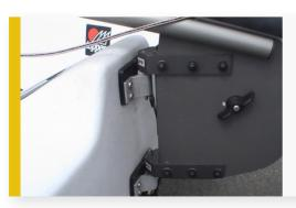
When the Rudder is attached ensure that it is fully engaged on to the pintle and gudgeon so that the retaining clip is able to spring out to hold the rudder in place.
