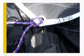
Attach the sheets to the clew (marked "C") with stopknot.
