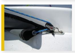
Then through the eyelet at the back of the sock. Feed it up the sock to the mouth of the chute.
