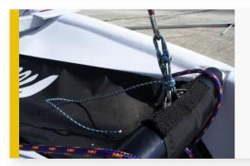
Having pulled the mast upright secure the forestay to the eye on the black bar at the chute mouth. Leave a long tail.
