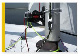
Make sure you are still head to wind. Raise the jib by pulling the halyard and cleating off at the base of the mast.
