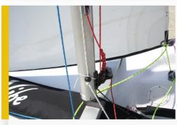
The Tail is kept next to the mast by tucking the ball under the elastic loop at the base of the mast.
