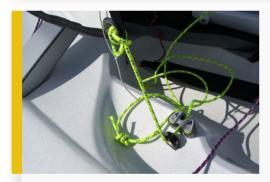
Attach the jib sheets to the clew of the jib with stopknot.
