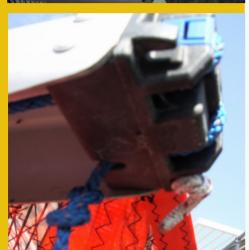
Before raising the sail, insert the slug at the back of the sail into the track on the boom.
