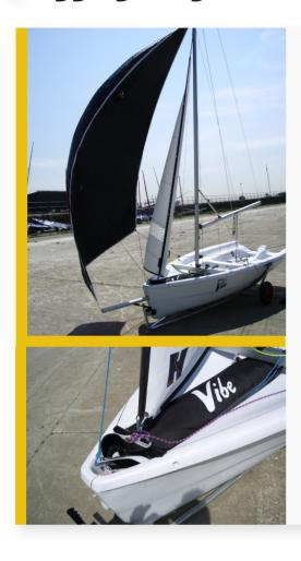
You should now be able to pull the gennaker down into the chute, ensuring that it does not snag around the poleend or under the bow.
