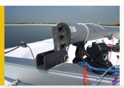
Fix the base of the mast to the mast step on the cross beam with the pin and ring from the mast step.
