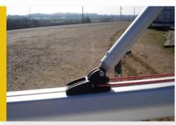
Fix the gnav strut to the carriage on the top of the boom. The carriage should already be fixed to the boom for you.
