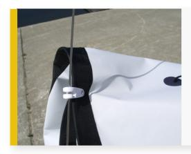
Lock the jib hanks onto the forestay, by inserting and twisting. Then, continue to feed the jib hanks onto the forestay.
