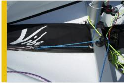
Lead the end down through the block at the front of the centerboard case. Round the back first (i.e., feed forward from the back of block).
