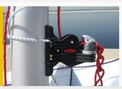
Having fixed the boom and gnav to the mast, thread the gnav control line from the fitting at the front of the boom through the cleat on the mast.
