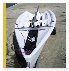
Position the boat head to wind away from any overhead power lines or other obstructions.
