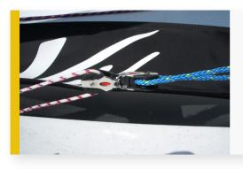
Then forward, around the free block located to the side of the gennaker chute (attached to the line that pulls the pole out).
