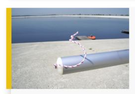
The tack line emerges from the forward end of the bowsprit. Tie a figure-of-eight knot about 6in /15cm from the end of this line and an overhand knot right at the end.
