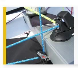
The gennaker halyard is entirely external to the mast. One end ties to the head (top) of the sail then passes through the top pulley block on the mast and to the small block on the beam.
