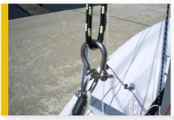
Attach jib head to the shackle on jib halyard. Pin downward.
