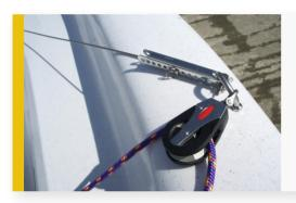
Untape all the ropes attached to the foot of mast. Attach shroud adjusters to the shroud eye each side - approximately the 7th hole down (approximately the middle of the adjuster). Subsequently, you can attach at the captive pin on the base of the plate.
