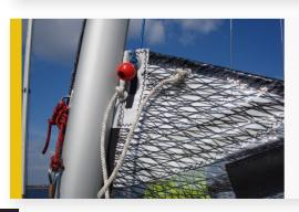
A good knot for tying the halyard to the head of the mainsail is a simple half-hitch with a stopper. This takes up less halyard than a bowline and fits snug to the headboard, allowing you to pull the sail right to the top of the mast (the luff bolt rope will stretch a little when you do this).
