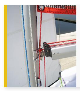
Cunningham - Take the tail attached to the gooseneck fitting and feed through eye in the sail then down through the cleat on the side of the mast. Secure this with a figure-eight knot.
