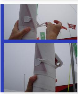
Wrap the sail up clockwise, so that the hook in the corner is on the outside. Once the sail is wrapped up, place the white loop on the hook to hold the sail wrapped up while the rest of the boat is rigged.
