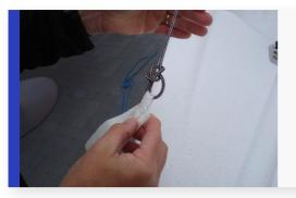
Tie the free end of the jib halyard from earlier onto the top of the jib using a bowline.
