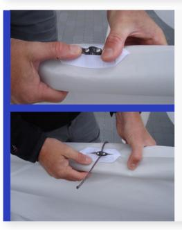
The block for the jib halyard should line up with the cut out on the luff tube. Pass one end of the jib halyard through the deckeye, and pull it towards the bottom of the mast.
