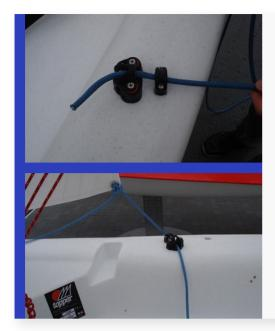
Pass the jib sheets through the cleats on the sides of the boat as shown.
