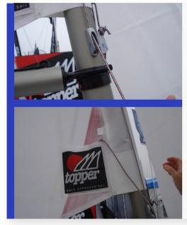
Pull the jib halyard until the jib is all the way up and the luff (front edge) is taut.
