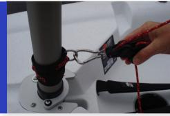
Clip the karabiner on the end of the kicker onto the metal ring at the bottom of the mast.
