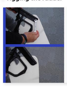
Attach the rudder blade to the rudder stock using the long bolts and nuts.
