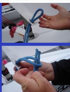
Attach the jib sheets to the jib by passing a loop through the metal ring in the clew of the jib.
