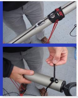
Take the free end of the outhaul towards the mast end of the boom, and pass it through the cleat on the top of the boom.
