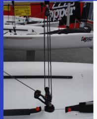
Tie one end of the mainsheet in the pulley on the boom.
