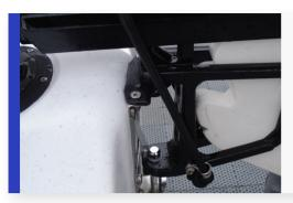
Line up the pins on the back of the boat and the rudder to attach.
