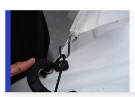
Clip the bottom of the luff of the jib onto the line on the bow.
