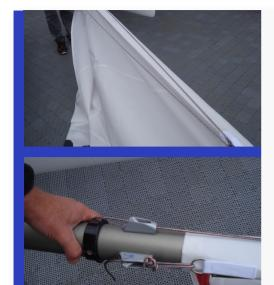
Lead the Jib Halyard to the other cleat on the mast and pass it through to secure it.
