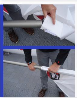
Slide the luff tube of the sail (front edge) over the mast until the end of the mast reaches the end of the luff tube.
