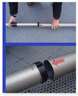
Lay the Upper and Lower mast on the ground. Insert the upper mast into the lower mast as shown.
