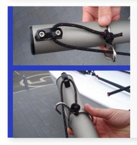
Tie the outhaul onto the hook on the boom, and then pass it through the block on the stern end of the boom.
