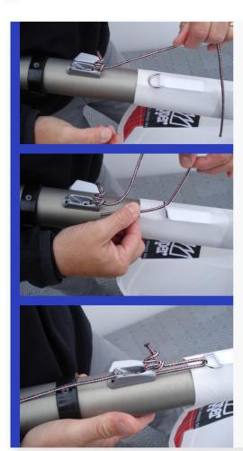
Tie the downhaul onto the pre-attached cleat on the lower mast. Pass the downhaul through the metal ring on the sail, and then back through the cleat. As shown.
