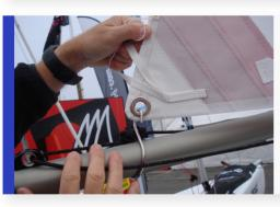
Unwrap the sail, and place the hook on the end of the boom through the metal ring in the clew of the sail.
