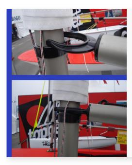
Place the gooseneck on the mast above the gooseneck ring, and push the gooseneck until it is around the mast fully.
