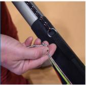
Take the end of the jib halyard with the figure eight and pull it to the bottom of the mast, and then secure this end on the mast.
