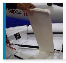
When ready to go sailing, insert the daggerboard into the slot.
