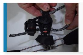
Pass the free end of the main sheet through the block on the hull, from the front of the boat to the back.
