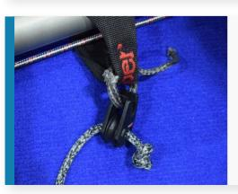
Tie the boom mainsheet block onto the topper strap in the middle using the short grey piece of dyneema.
