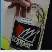
Pull the jib up using the halyard, and then secure using the cleat. Tuck the halyard into the pocket on the sail behind the topper logo.
