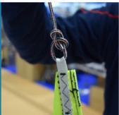
Tie the jib halyard from step 1.5 to the head of the jib.
