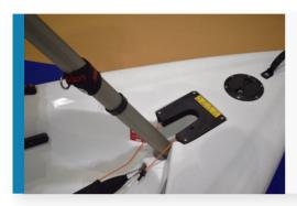
Place the mast foot in the hull and lift until the mast is vertical.
