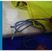
Attach the jib sheets. Fold the jib sheets in half, and then pass the loop through the metal eyelet in the clew. Pass the ends of the sheets through the loop and pull tight.
