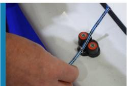
Pass the ends of the jib sheets through these blocks on the sides of the hull.
