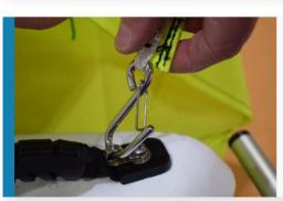
Clip the tack of the jib onto the P clip on the bow.
