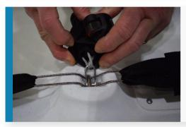
Tie the mainsheet block onto the hull of the boat as shown, with the cleat on the block pointing towards the stern of the boat.
