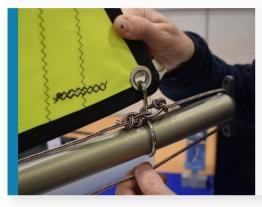
Unwrap the sail and hook the metal eyelet in the clew to the boom.
