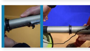
Tie one end of the downhaul onto the block near the bottom of the mast, then pass the other end of the downhaul through the ring on the sail.
