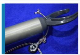
Tie the pulley onto the front end of the boom as shown, then pass the free end of the outhaul through the pulley.
