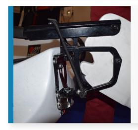
Attach the rudder to the stern by lining up the top and bottom pins. It can help to put downward pressure on the rudder and rotating the tiller back and forth.
