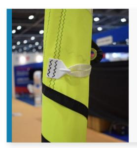
Wrap the sail up by passing it clockwise around the mast and secure the sail by hooking the white strap on the hook as shown. This keeps the sail secured while the rest of the boat is rigged. 8
