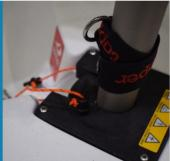
Secure the mast by pulling the orange lines to close the mast gate.
