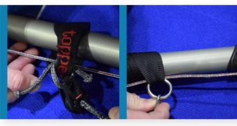
Pass the free end of the outhaul through the topper strap in the middle of the boom (left), then through the kicker strap and the block near the front end of the boom (right).
