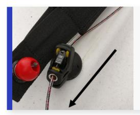
Pass the halyard through this pulley in the middle of the deck, from front to back (in the direction shown).
