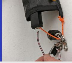
Pass the halyard up the spinnaker bag until it comes out of the front opening.
