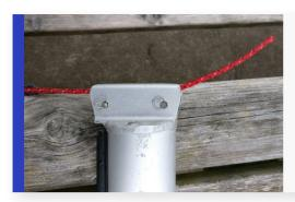
The Topaz Race R2 has a tracked mast with a halyard as standard. Insert the upper mast into the lower mast so that the track lines up. Then pass the red halyard through the top of the mast from the back (with the track) to the front as shown.
