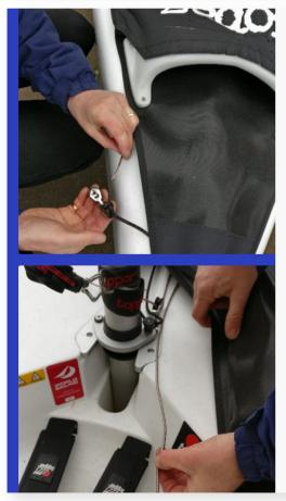
Pass the halyard through this pulley, found underneath the spinnaker bag at the bow. Then pass the halyard back underneath the bag towards the stern.
