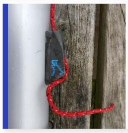
Secure the end of the halyard in the cleat at the bottom of the mast on the front side.
