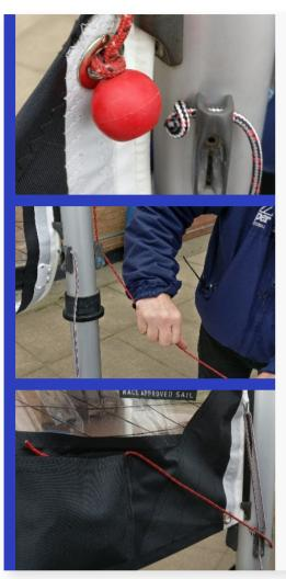
Place the head (top) of the sail in the mast track and pull the free end of the halyard to raise the sail. Once the sail is at the top of the mast, the halyard can be coiled and placed in the velcro pocket near the tack of the sail.
