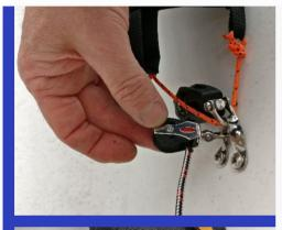
Pass the halyard through the pulley on the starboard side of the deck and then through the eyelet on the back of the spinnaker bag. 7
