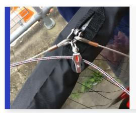
Pass the other end of the halyard through the pulley on the upper fitting on the mast.
