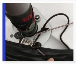
Pass the end of the spinnaker halyard through this pulley at the base of the mast.
