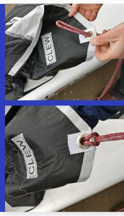
Using the spinnaker sheets, pass a loop through the eyelet on the clew. Then pass the ends of the sheets through the loop and pull tight to secure it.
