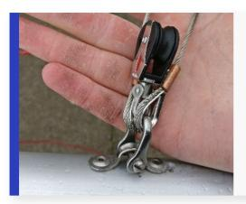
If you intend to use the asymmetric spinnaker, please attach the shrouds and spinnaker halyard pulley to the upper of the two fittings on the front of the mast. 6
