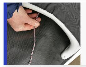
Tip: tying one of the red balls to the end of the halyard can make it easier to feel through the fabric and push through to the bow opening.
