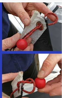
Pass a loop of the halyard through the eyelet at the top of the sail. Pass the red ball through the loop and pull it tight to secure it.
