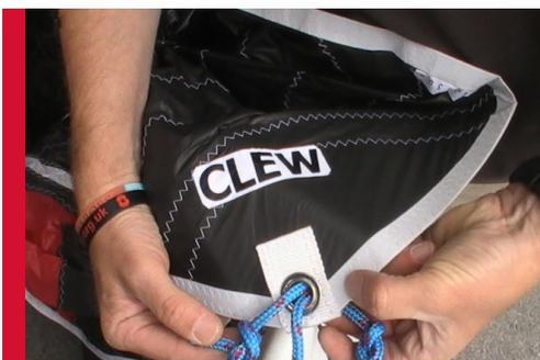
Tie the spinnaker sheets onto the CLEW of the spinnaker.
