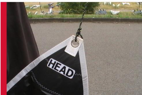
Tie the end of the halyard that you tied around the furler bar at the beginning onto the HEAD of the spinnaker.
