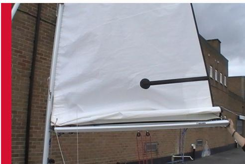
Release the main halyard from the cleat, and uncleat the gnav, and then pull on the reefing line. The foot of the sail should fold up so that the sail area is reduced.
