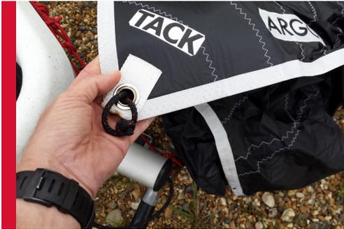
Then tie the spinnaker pole to the TACK of the spinnaker.
