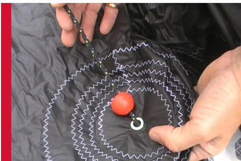
Then re-attach red ball to spinnaker halyard on the other side of the sail.
