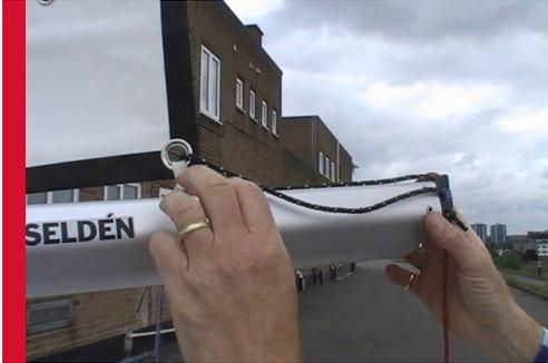
Pass the outhaul through the eyelet in the clew, and then back to the end of the boom, where the end of the outhaul should be cleated.
