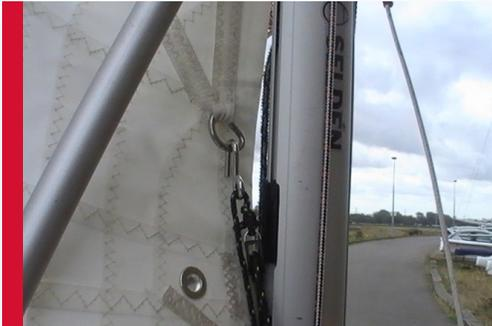
Hook the downhaul onto the sail, ensuring that it is not twisted before applying any tension.
