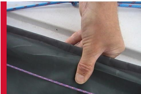
Pass the line up the chute, feeling for the ball inside, until it reaches the opening at the front.
