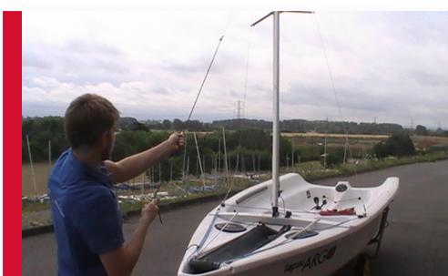
Pull the mast up using the forestay. To make it easier, someone else can lift the top of the mast.
