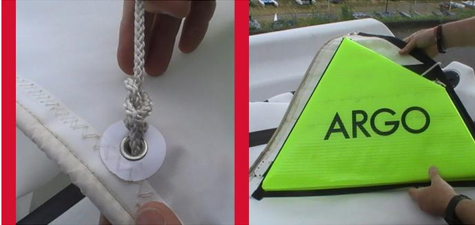
1 Tie the flotation panel to the top of the mainsail by passing the white lines through the eyelets in the sail and secure with a figure of eight knot.
