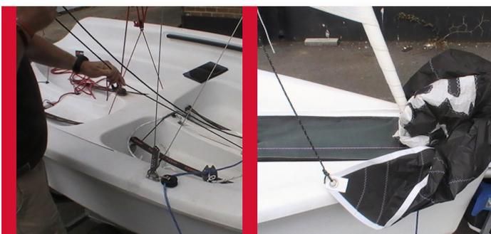
Pull on the end of the spinnaker halyard coming from the end of the spinnaker chute within the boat in order to pack the spinnaker into the chute.
