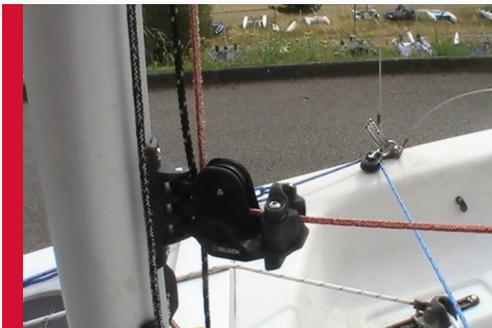
Having fixed the boom and gnav to the mast you can thread the gnav control line. This comes out from the boom at the front, and then feeds through the swivel cleat on the mast.
