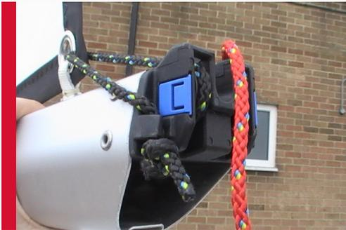
Pull on the red reefing line so that it comes out of the boom some way.
