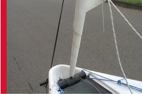
Furl the jib by pulling the thin line, so that it ends in this position.
