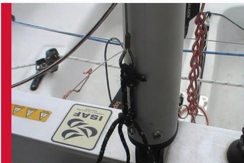
Once the rig tension has been applied, the forestay can be moved back from the bar at the front and then tied off to the mast.
