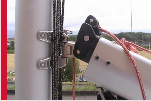
Attach the boom onto the mast with the pin on the lower of the two fittings. Remember to put the pin in from the top and flip the pin end over.
