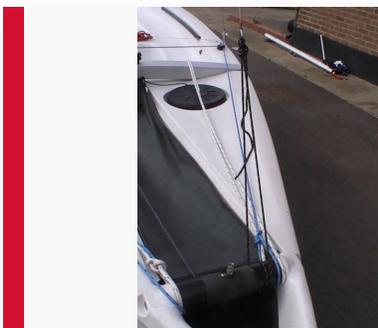
Having pulled the mast upright, secure the forestay around the stainless steel chute mouth bar.
