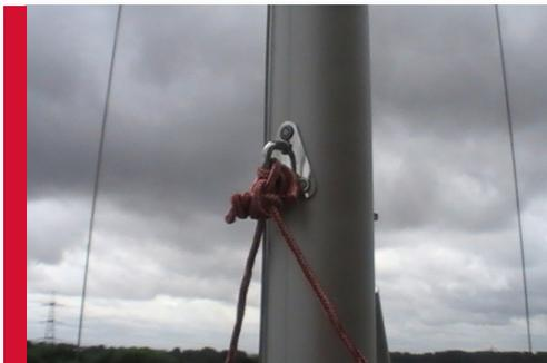
Now tie the lowers onto the fitting on the mast.
