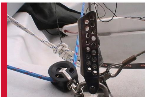
Attach the shroud adjusters to the shroud eyes each side, on approximately the 5th hole down on the stern side.
