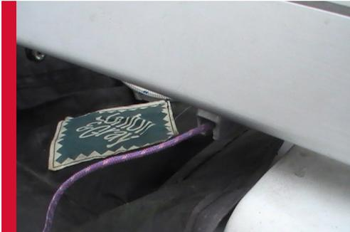
Cleat the jib furler off in this cleat underneath the crossbeam.
