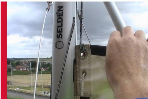
3 Raise the sail by placing the bolt rope in the cut out of the mast just above the boom, and then pulling on the halyard.
