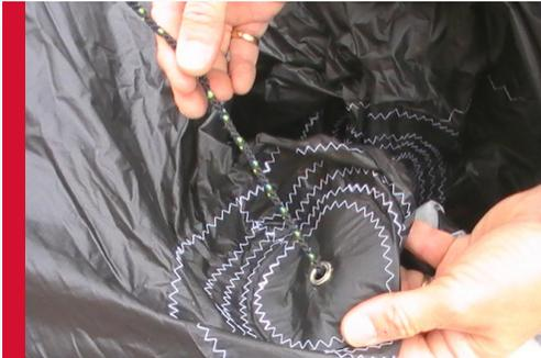
Temporarily remove the red ball from the spinnaker halyard. Then pass the end of the spinnaker halyard through the eyelet in the sail as shown.
