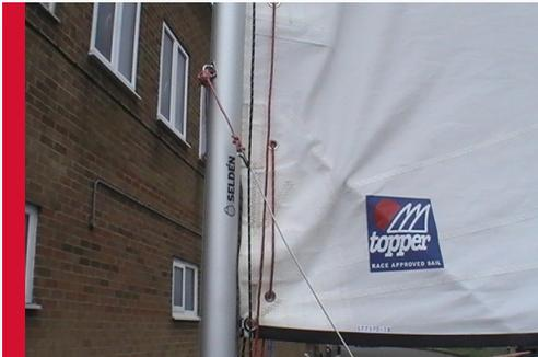
Use a similar system, with the end of the reefing line at the mast end of the boom, on the luff of the sail.
