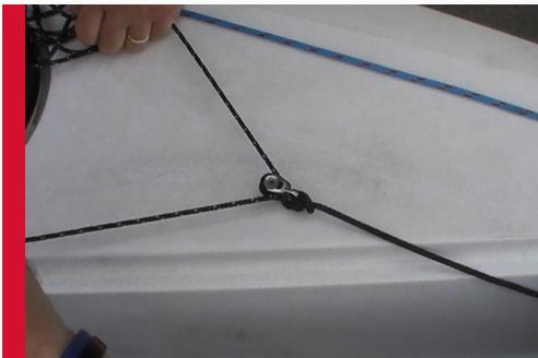
Take the free end of the halyard through this cleat; it is underneath the spinnaker chute, and it may need to be moved for the pulley to be exposed.
