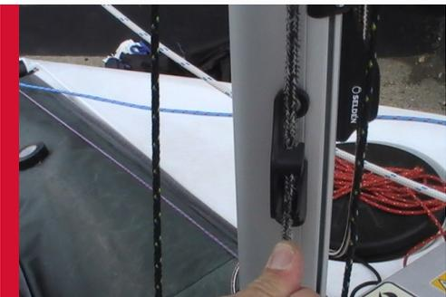
4 Cleat the main halyard in the cleat on the left of the mast, in order to make sure that the sail is at the top of the mast. This is done by holding the halyard just above the cleat and then pulling away from the mast at 90 degrees. Then re-cleat the halyard until the sail is at the top of the mast.
