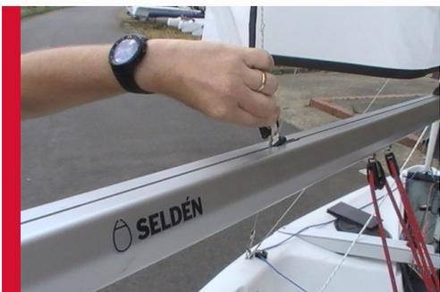
5 Insert the slug at the clew of the sail into the cut out in the boom, and slide it along to the end of the boom.
