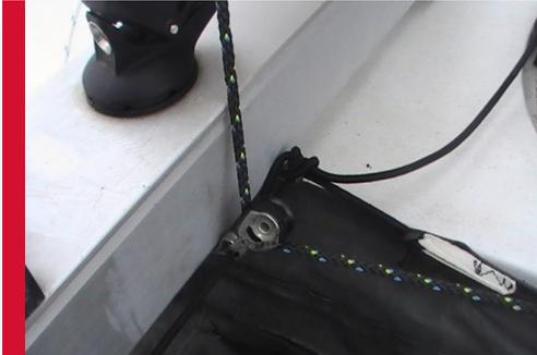
Take the other free end of the halyard and take it through this pulley on the front of the cross beam.
