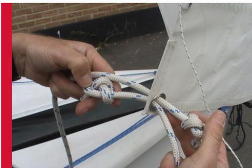
Tie the jib sheets onto the eye on the clew of the jib.
