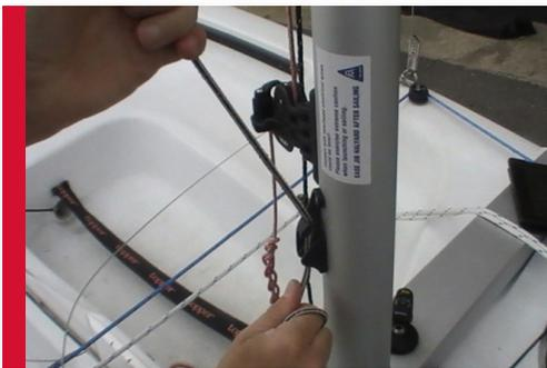
Pull the jib halyard in order to raise the jib, and then cleat the halyard off on the right side of the mast. In order to apply the most rig tension, sweat the jib halyard as shown.
