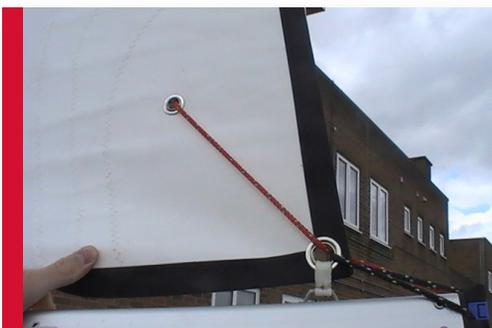
Feed the reefing line through the eyelets in the leech of the sail.
