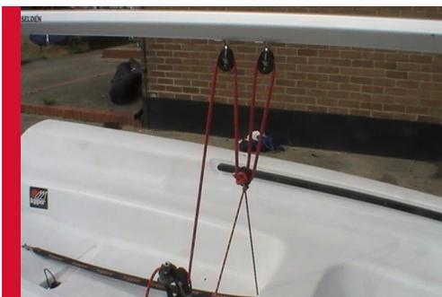
Now thread the mainsheet. Starting from the centre cleat on the hull (NB: ensure the ratchet clicks when the rope is pulled in), go up to the rear block, and thread the line from back to front. Then go to the pulley on the top of the centre block, and thread it from back to front. Then go to the front pulley on the boom, and thread it from front to back.
