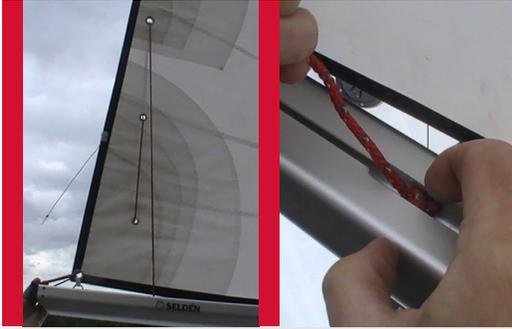
From the top eyelet, the reefing line comes back down to the boom.
