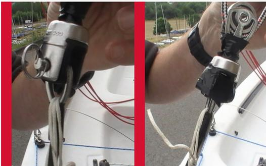
Do the same for the head of the jib onto the furler on the jib halyard. Again, wrap some tape around it.
