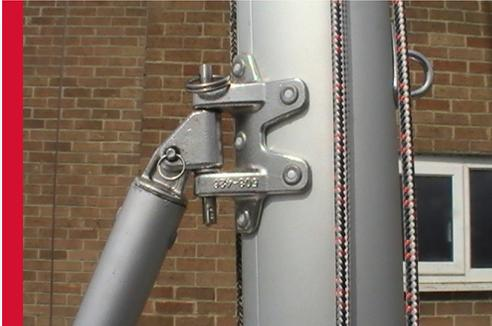
1. Next attach the strut to the upper fitting on the mast. Ensure the toggle is correctly orientated as per the Selden/Super Spar info sheet.
