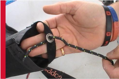
Pass the halyard through this eyelet in the bottom of the spinnaker chute.
