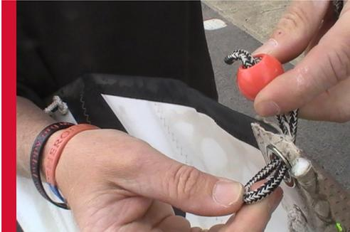
2 Tie the free end of the main halyard to the eyelet on the top of the mainsail.
