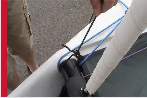
Tie one end of the Spinnaker halyard around the front furler bar.
