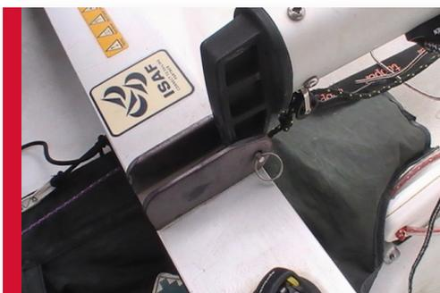
Fix the base of the mast to the mast step on the cross beam with the pin and ring from the mast step.
