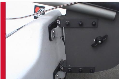
When the Rudder is attached, ensure that it is fully engaged on to the pintle and gudgeon so that the retaining clip is able to spring out to hold the rudder in place.
