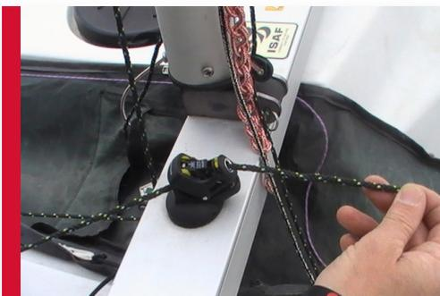
Take the halyard through this pulley that is mounted on top of the crossbeam.
