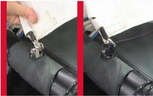
Attach the foot of the jib to the furler at the front of the boat. Ensure the furler is fully wound up.
