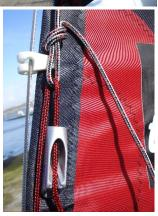
Attaching the jib sheets, the Topaz 14 uses a 2:1 purchase jib sheet system running through 2 eyes in the sail.
