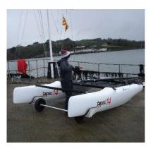
Once the mast is fully upright the forestay is loosely tied off to the furler drum. This allows the mast pin to be removed so the mast can rotate.
