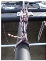
The dynema lines attached to the front of the pole are to stop the pole being pulled up when sailing. In order to tension these correctly the help of a second person is needed.
