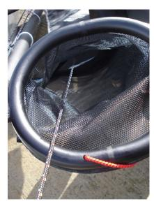
The rear of the sock can now be secured by with the lines attached to the loops, one side ties around the mast foot and the other ties around the beam passing through the eyelet on the trampoline. These do not need to be pulled tight as they are only there to support the sock. Also the sock will move while sailing so you need to allow for that to take place.
