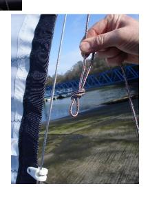
Take the tail from the forestay/jib tie down through the loop in the halyard and down through the cleat on the jib.
