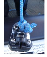
Feed the jib sheet through one eye on the sail and then back down and through the cleat.
