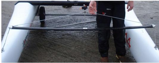
The mast can now be lifted back do the mast foot can be fitted to the ball on the crossbeam (the securing pin can be inserted).
