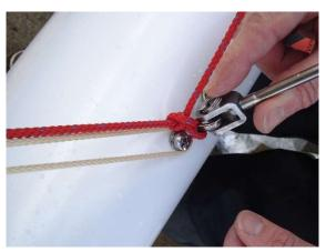
Before the halyard for the spinnaker can be treaded up the halyard turning ring at the rear of the trampoline needs to be fitted and the sheet blocks.
