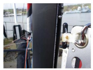
When the sail is fully hoisted, the halyard is secured in the cleat on the side of the mast and the tail of the halyard stored in the pocket on the trampoline.
