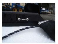
When the trampoline is central it can be laced to the rear beam. Attach the tensioning line to one end of the rod in the trampoline with a bowline.
