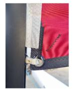
The Downhaul will need to be treaded the first time you rig the Topaz 14 it can then be left attached to the sail and hooked back on to the mast each time.
