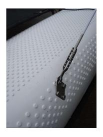
In preparation to raise the mast you will need to attach the striker bar to the bow of the hull. The furler drum is attached the screw fitting at the centre of the striker bar.
