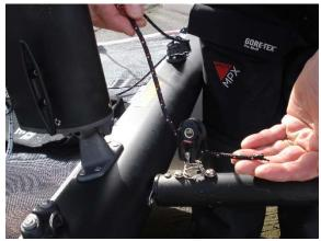
The line then threads through the double block attached to the tack line (this pulls the sail to the end of the pole.
