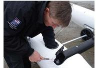
Once the hulls have been bolted together refit the hatch covers.
