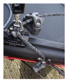
Slide the car along the track till the figure of 8 knot reaches the cleat, this should stop between 5 and 10 cm short of the end stop. If the car is hitting the end stop, move the position of the knot to prevent this.
