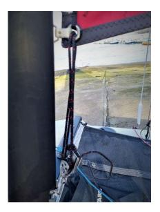
The mainsheet is simply hooked in to the eye at the back of the main sail
