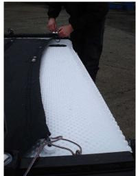
The side lines can now be pulled tight at the rear beam to tension then. When tight secure the line to the metal loop (using 2 round turns and a half hitch). Leave a long tail as this is used to tension the trampoline at the back by feeding through the metal ring on the trampoline.
