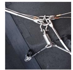
The rigging can then be attached to the mast NB please ensure all shackles are securely tightened.
