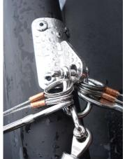
Also if you have the trapeze kit you can now fit the mast head halyard pulley. This is tied off to the metal eye near the top of the mast with a round
