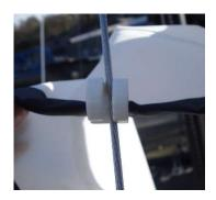
When the jib is fully hoisted untie the two parts of the halyard. Tie an overhand knot loop in the end of the section attached to the top of the jib (you will only need to do this the first time you rig). The rope you have untied is stored in the pocket on the trampoline until you need it to drop the jib after sailing.
