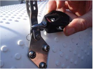
To thread the spinnaker halyard, first secure one end to the end of the pole so you do not lose it up the mast.
