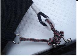
The central tie can now be fitted to the small metal loop on the hull midway between the beams.
