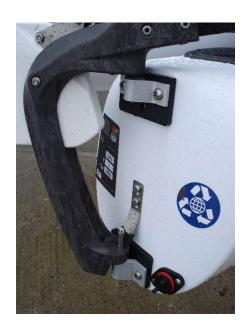
The connector cross bar and tiller extension are connected together using the UJ, the cover plates need to be clipped in place to ensure the joint cannot come apart.
