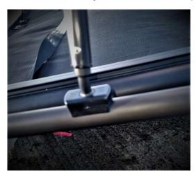
When on the water the rudder blades are pushed down and secured in place by putting the bungee loops over the stainless steel arm.
