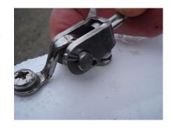
When the striker bar is fitted correctly the wider rounded side will face forward.
