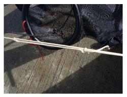
The Line attached to the shoot mouth is tied off to the bow fitting on the port side as well, this line is to hold the shoot mouth up and make it easier to launch and retrieve the spinnaker.
