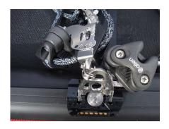
Tie 2 figure of 8 knots in the mainsheet (approximately 1m and 0.75m in from the end of the mainsheet, these may need to be adjusted latter), 1 is to limit the amount you can sheet out and the other is to limit the travel of the car so it does not hit the end stop on the crossbeam.
