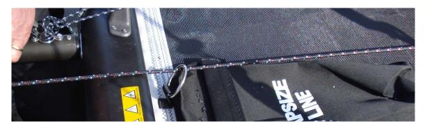
The halyard can now be fed through the spinnaker sock (it is easier to reach down the sock if it is not attached to the pole of the boat). When you have
