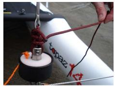
With the mast up the Trapeze wires can be secured to the elastic.
