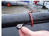
Attach the shroud adjusters to the plates on the hulls and the shrouds the approximately the 4<sup>th</sup> hole down.
