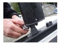
Once the pin has been removed the rig tension can be pulled on unsing the forestay,
