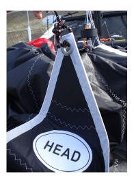
Now work down the back edge of the sail to the Clew to attach the sheets.
