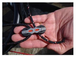
The halyard is then lead back through the cleat on the cross beam, to the ring by the rear beam and forward to the metal ring at the front of capsize line pocket (remember to feed the line under the jib sheets).
