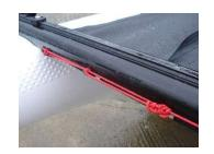
The side tensioning lines can now be attached, first attach the loop to the metal eye on the rear cross beam and take a couple of turns through the plastic ring on the trampoline side rope, then tie off loosely.
