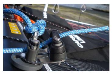
Pass the jib sheet across the trampoline and through the other jib cleat, through the other eye on the jib sail and then tie the end to the bridge on the cleat.
