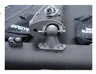
In order to raise the mast you will need assistance, one person will need to lift the mast from the back of the boat. They walk forward while the other person pulls up on the forestay or trapeze wires.
